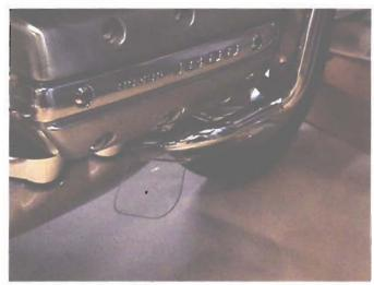
INSTALL RAIN SHIELDS UNDER CASE GUARDS, INSERT SHIELD IN A FRONT TO BACK MOTION. ( 06 model back to front) CLIPS ARE GUARANTEED, RETURN SHIELD with \$6.00 shipping for REPAIR OR REPLACE.
