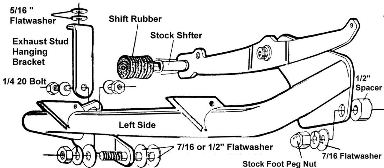
7. Finally, fasten the exhaust stud hanging brackets to the front side of the slotted tabs on the floorboard supports using the 1/4 20 x 3/4" bolt sets. (On GL1000 only, the hanging bracket may require mounting to the backside of the slotted tabs.) Tighten all nuts and bolts securely.
