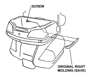
3. Remove the original center molding from the trunk.
