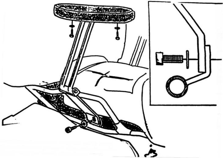
**5. Fasten the armrest pads to the mount assemblies as shown, using the 1/4-20 x 3” bolts and flat washers provided. Adjust their position forward or back (to suit the passenger’s riding style and/or position of the trunk if you have a relocation kit installed), and then securely tighten these four bolts.**
