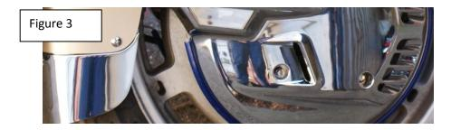
5. Put on the new rotor cover using the original bolts. Replace in reverse order.
