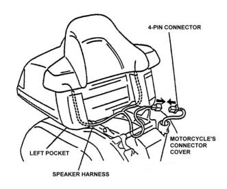
**17.** Secure the harness with the two wire ties in the areas shown.
