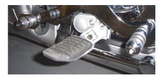
3. Install shifter slot over shifter peg.
