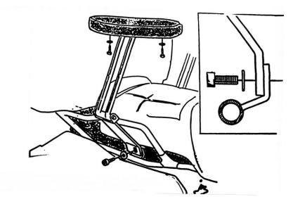
5. Fasten the armrest pads to the mount assemblies as shown, using the <sup>1</sup>/<sub>4</sub>-20 x 3" bolts and flat washers provided. Adjust their position forward or back (to suit the passenger's riding style and/or position of the trunk if you have a relocation kit installed), and then securely tighten these four bolts.
